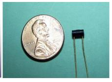
Wire wound resistors are ideal for compensating strain gage transducers: They offer the necessary accuracy, and perform reliably at high temperatures. They are designed so that resistance value does not change, or changes in a controlled manner, over different temperature.
